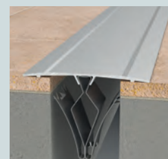
W-90 installed over 50mm joint width using large clip option.
