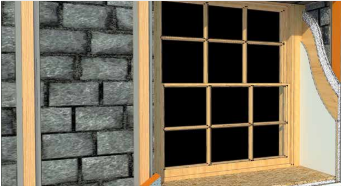
Image showing Spacetherm ® WRB applied internally to a reveal on an existing external wall structure.
