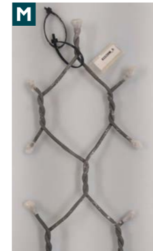
Test Specimen, before and after Salt Spray Test (ISO 9227)
