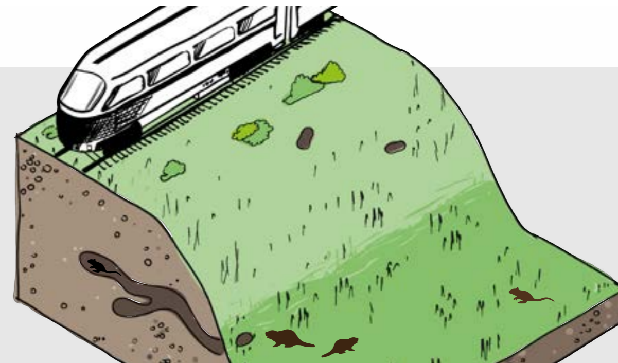
Other burrowing animals such as badgers dig lairs with multiple entry points. If those extensive tunnels are dug under road/railway embankment, those leave a high risk of subsidence to the bank and road/rail track.
