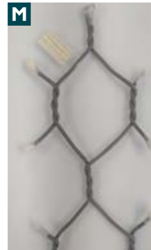
Test Specimen, before and after Salt Spray Test (ISO 9227)
